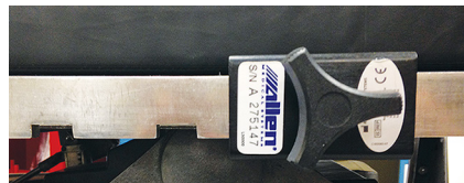
Figure 2b: Move the clamp to the right, away from the slots in the rail
