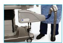
4. Loosen knob on the rail clamp to remove ALLY II. Lift using blue handle and flexible arm. Place the ALLY II and the rail clamp in the cart for storage.
